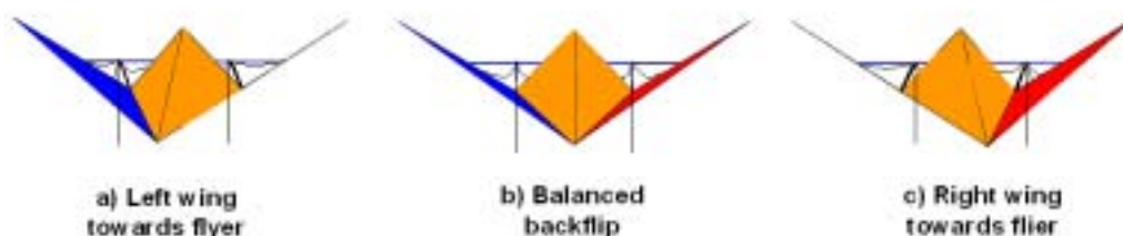
Figure 33 Balanced and unbalanced backflips Views are from flyer's side.
