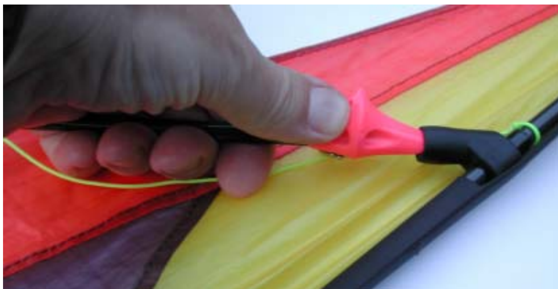
Figure 47 Using a kite mate spar remover
